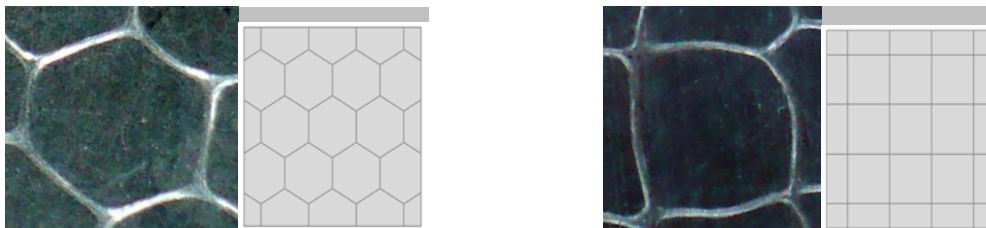
Figure 2: Final shapes of the rod cells with unidirectional carbon fibres and their distribution in a hexagonal and rectangular core of the RVE
